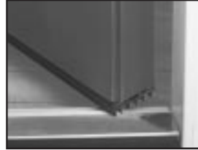
Vinyl 6-finger bottom weather-stripping fits securely into the threshold channel for a weathertight seal and can be replaced without removing the door. Advanced foam compression perimeter weather-stripping (not shown) provides an airtight seal to keep out water and air.
